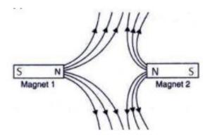
ii) Magnet 2 is weaker because its field lines are smaller than that of the magnet.
